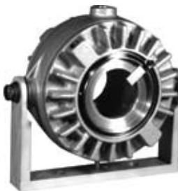
The air shaft seal **TRANSMITS AIR** from the air supply to the rotating members of air clutches and air brakes making possible new applications of air clutches and air brakes previously considered impractical for closed-end shafts. The **SLIP-ON INSTALLATION** eliminates long rifle drilling of air passages in shafts and permits easy installation.
