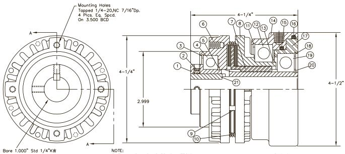
1. Torque Capacity @ 80psi = 350 in-1b
